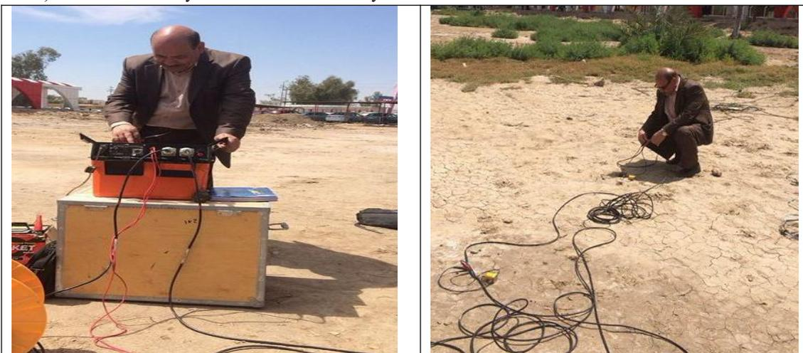
Plate (1. a,b) Shows ( $V_p$  and  $V_s$ ) refraction field work for study site.
