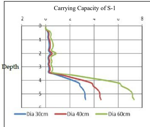
**Gambar 4a.** S-1 Borepile Capacity Chart
