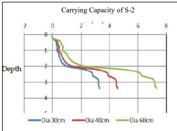
**Gambar 4b.** S-2 Borepile Capacity Chart
