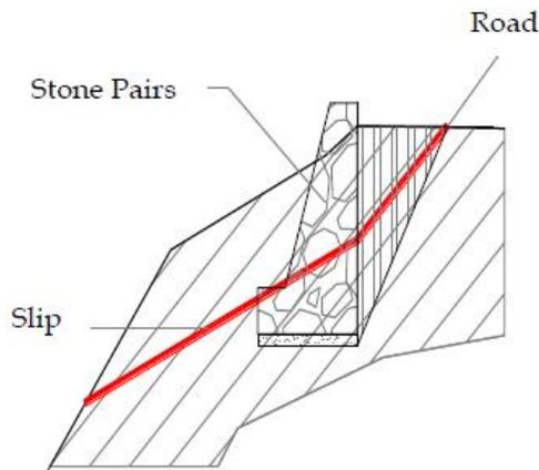
**Figure 7.** Reconstruction of retaining wall for handling Nagrak road avalanche
