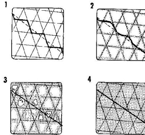
**Figure 5.** Slickenside patterns at each stage of weathering generally along a segment
