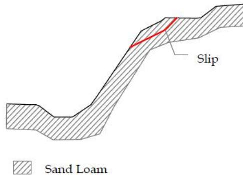
**Figure 6.** A typical stratification pattern that has collapsed on the slopes of Nagrak Street
