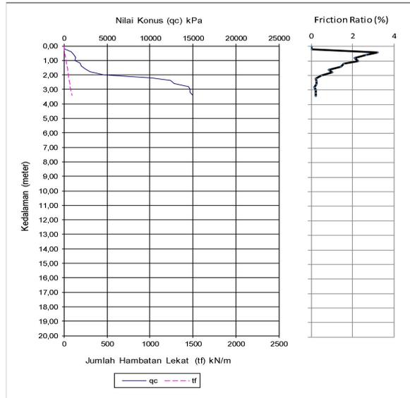
**Figure 2.** Dutch Cone Penetrometer Graph S-1
