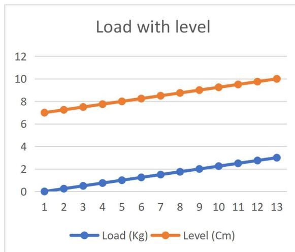
From the measurement results, it can be concluded that if the object load is 3 kg, the water level will be 10 cm, so this shows that every increase in object load is 0.25 kg, the water level rises to 0.25 cm. Or if it's more detailed then every 100 grams the water level rises 1 dm.
