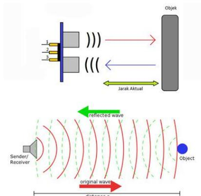
Picture 2. How the ultrasonic sensor works
