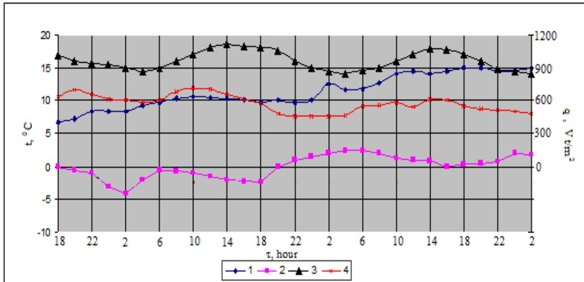
Fig. 1: Diagram of Air Temperature and Heat Flux Changes During the Observation Period: 1 - Temperature of Air Inside the Production Room; 2 - Temperature of External Air; 3 - Heat Flow through the Control Section of the Wall; 4 - Heat Flow through the Ventilating Wall Panel
