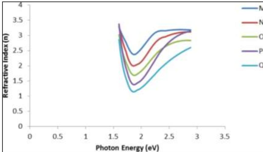
Figure 5: Refractive Index against the Photon energy (eV) for (PEO/PVA) composites thin films of different concentrations of CoCl<sub>2</sub>.
