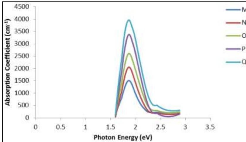
Figure 2: Absorption Coefficient for (PEO/PVA) Composites Thin Films of different Concentrations of CoCl<sub>2</sub>.
