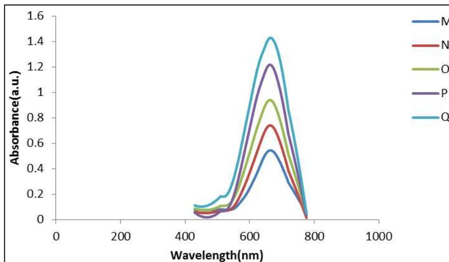
Figure 1: Absorbance for (PEO/PVA) composites thin films of different concentrations of  $\text{CoCl}_2$ .
