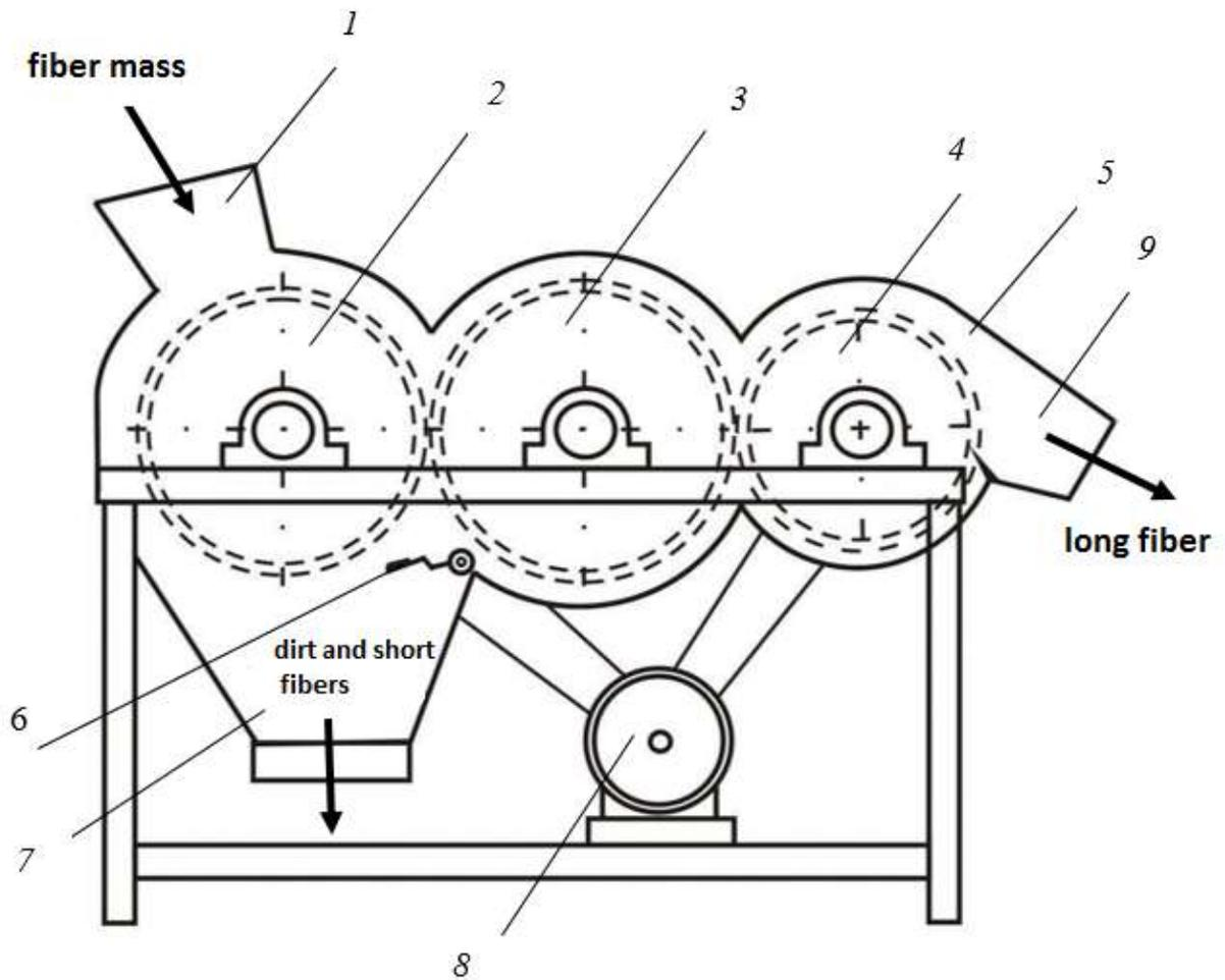
Figure 2: Schematic Diagram of a Spinning Cotton Fiber Separation Device
