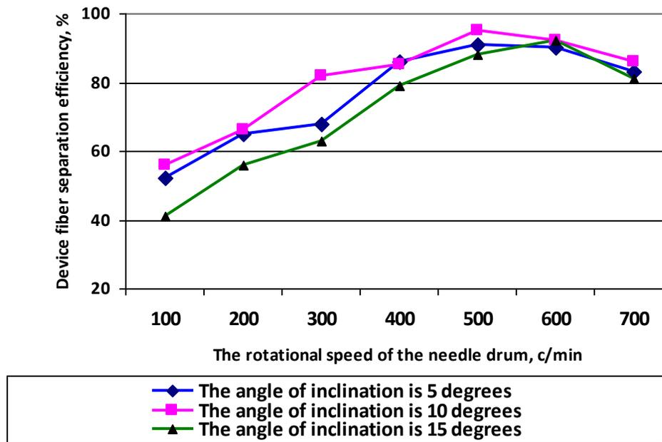
Figure 4: Graph of Dependence of Needle Drum Rotation Speed on Device Separation Efficiency at Different Slope Angles
