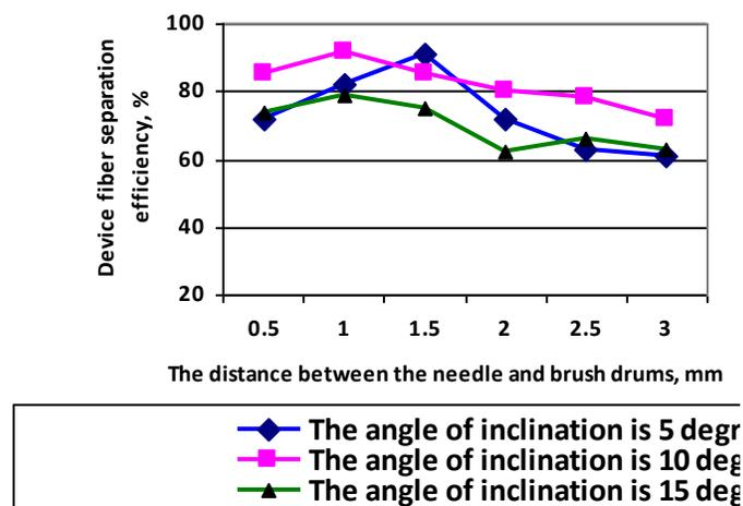
Figure 3: Graph of the Distance between the Drums at different Slope Angles as a Function of the Separation Efficiency of the Device
