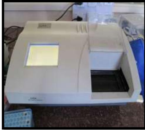
Fig. 8: Micro-plate reader machine
