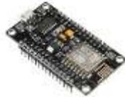
Figure 4: NodeMCU
