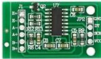
Figure 5: HX711 A/D converter
