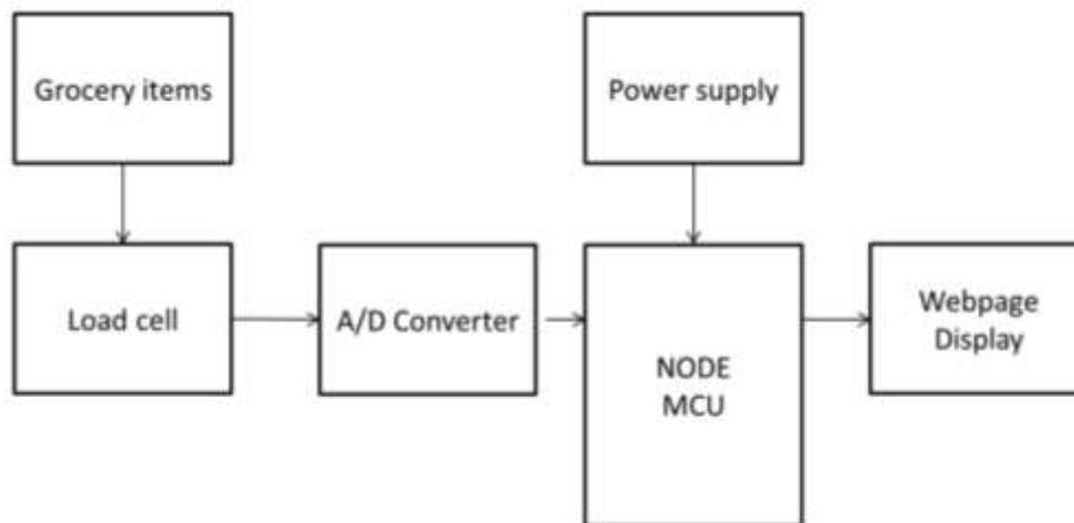
Figure 1: Block diagram of a home grocery management system using IoT
