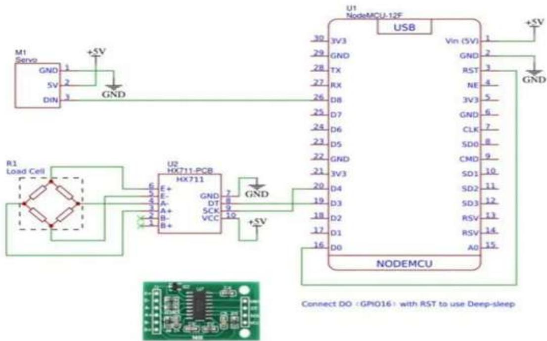
Figure 2: Internal circuit diagram of a smart kitchen shelf
