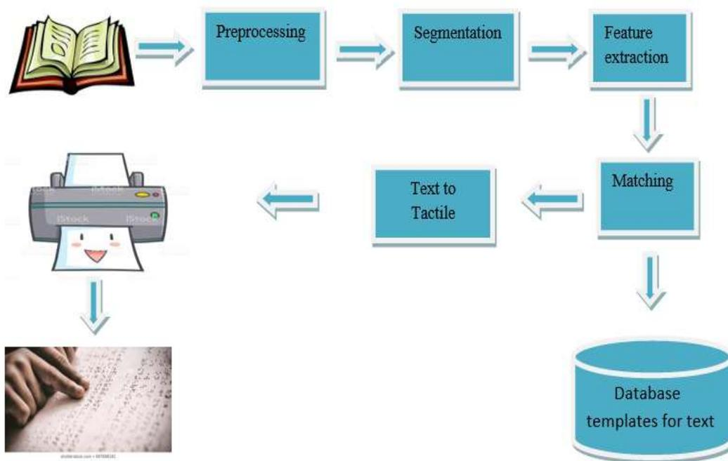
Fig. 3: System Architecture
