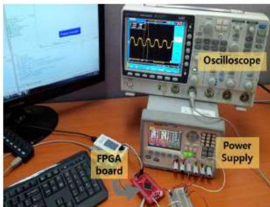
**Fig. 2** Setup for experimental measurements
