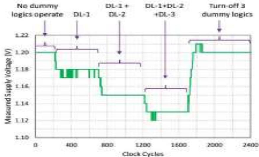
**Fig. 5** Results of voltage drop measurement
