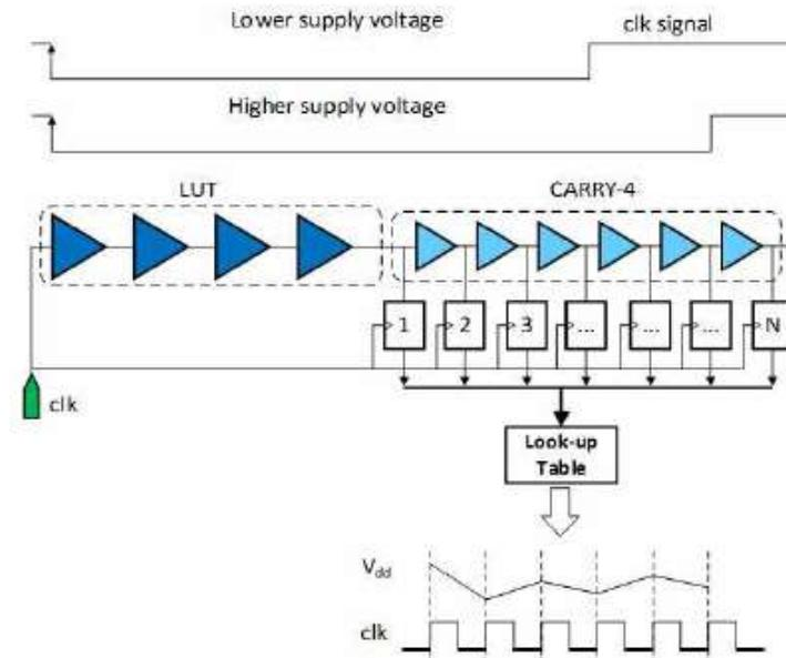
**Fig. 1** A supply voltage sensor schematic
