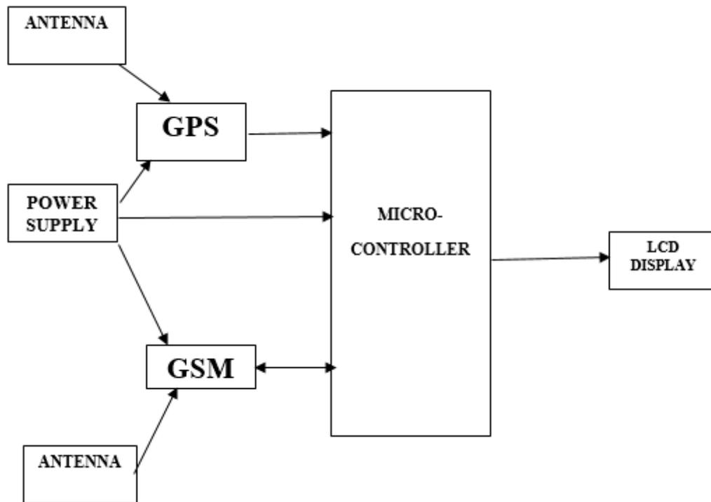
**Figure 1: Block diagram of System design**
