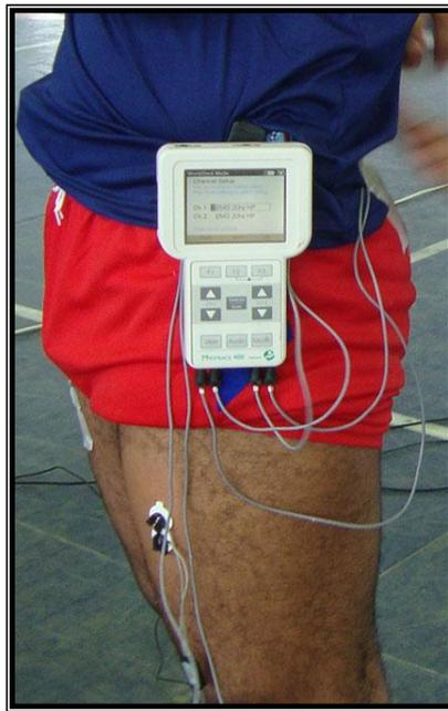
Figure (1) EMG device and surface pickups
