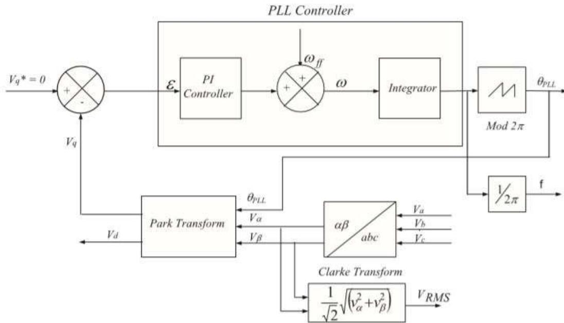
Figure 16. Block diagram of grid supervising model based on PLL
