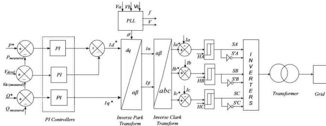
Figure 9. Adaptive hysteresis current control block diagram
