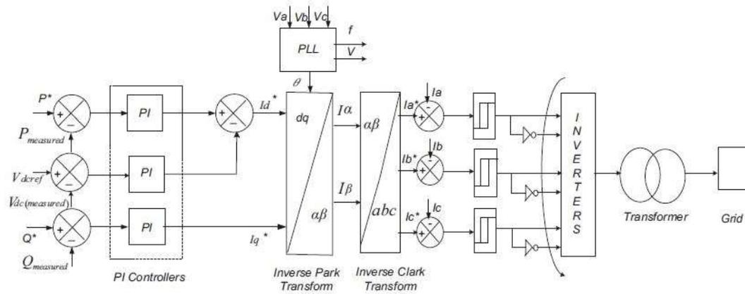
Figure 6. Control of Synchronous voltage oriented using PI controllers.
