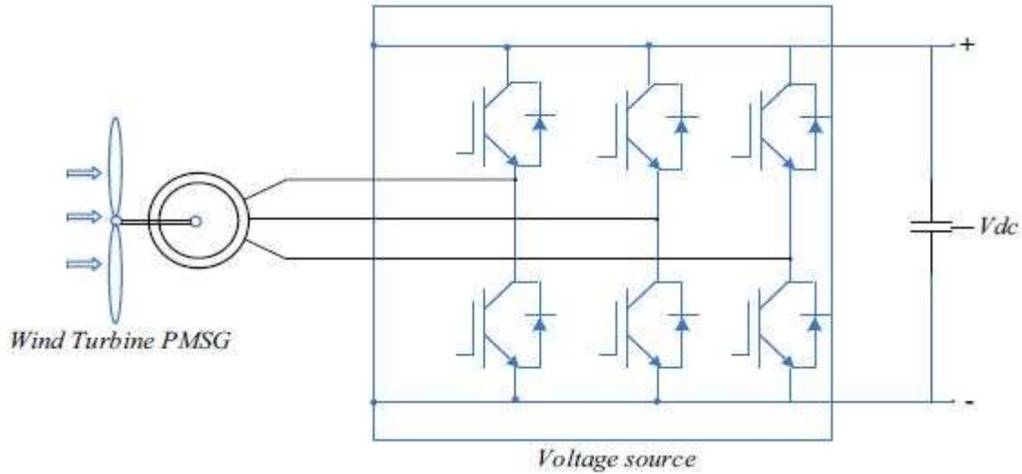
Figure 2. WECS organization of machine side converters.
