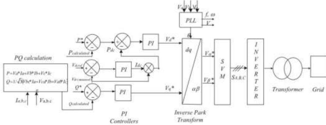
Fig. 10. Direct power control with space vector modulation.
