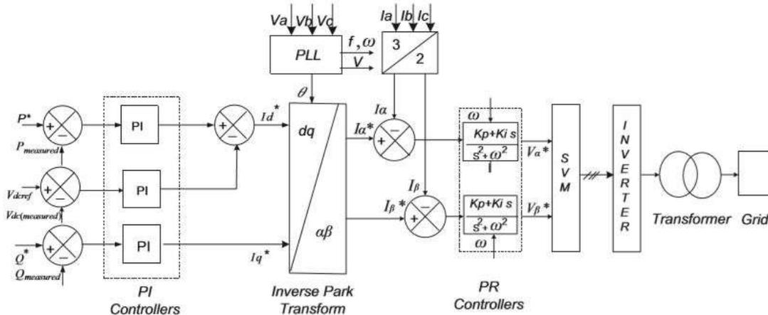
**Figure 7. Stationary VOC with proportional resonant controller.**
