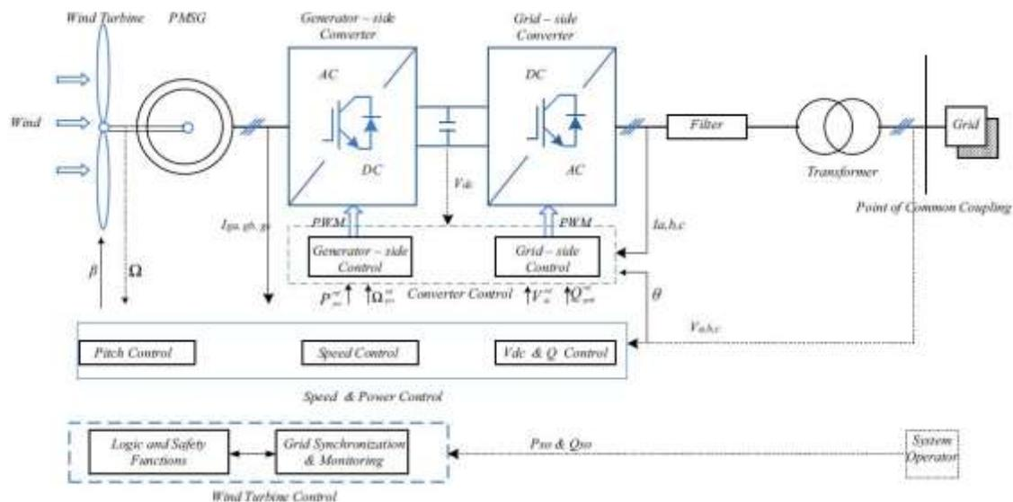
**Figure 1. WECS overall controlling levels.**
