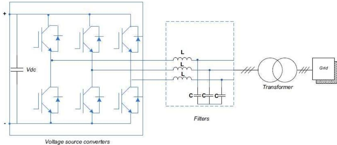
Figure 5. WECS grid side converter organization
