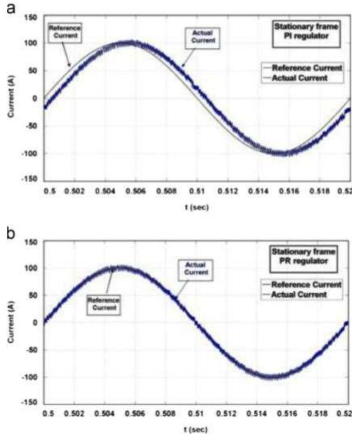
**Figure 15. Steady state operation for stationary frame: (a) PI current controller (b) PR current controller applied to an R-L load**
