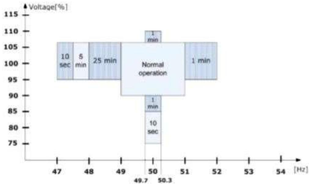
Figure 18. Voltages versus frequencies plot for a wind turbine
