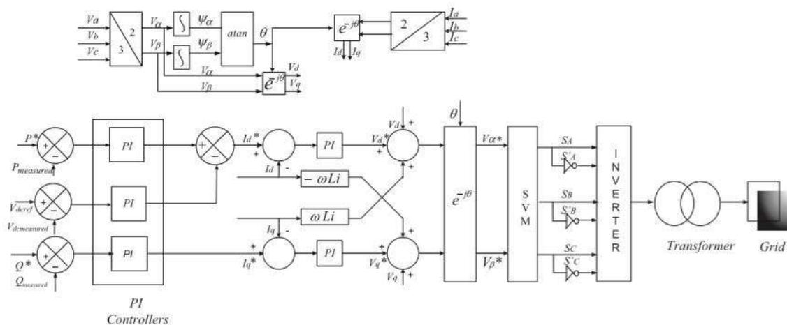
Figure 8. Synchronous virtual flux oriented control with PI controller.
