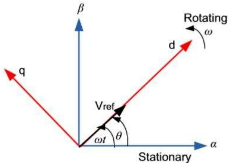
Figure 17. Synchronous rotating reference frames.
