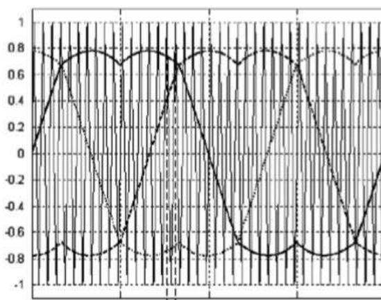
Figure 14. Triangular carrier SVPWM.
