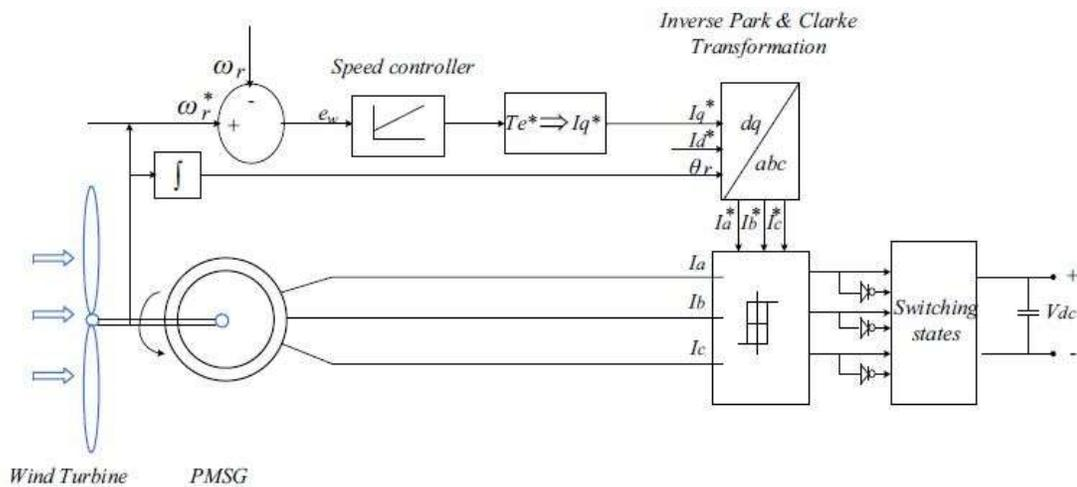
**Figure 3. The generator side converter field oriented controlling strategy block diagram**
