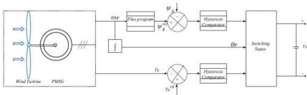
**Figure 4. Generator side converter direct torque controlling strategy block diagram**
