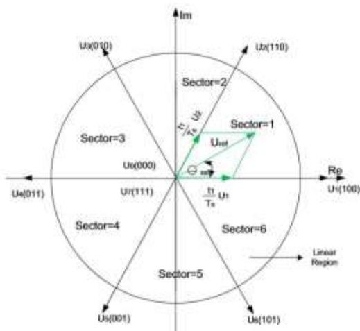
Figure 12. Representation of inverter states in space vector.
