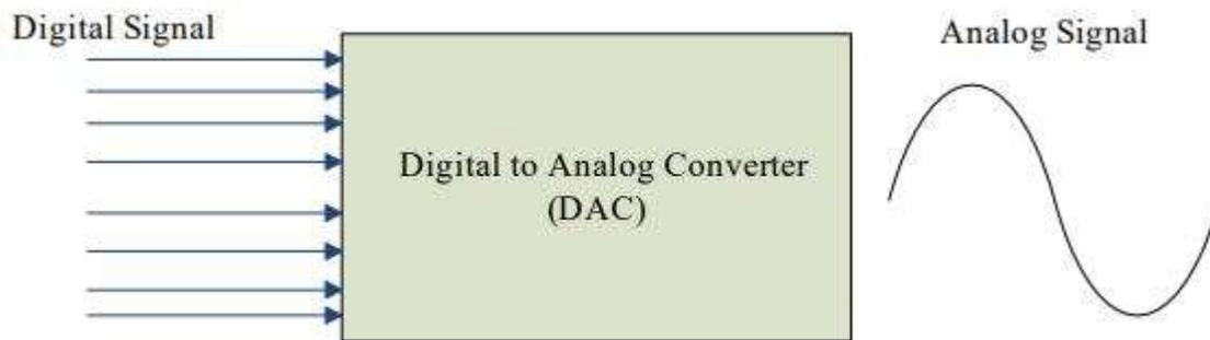
**Figure 1:** Digital to Analog converter block diagram.
