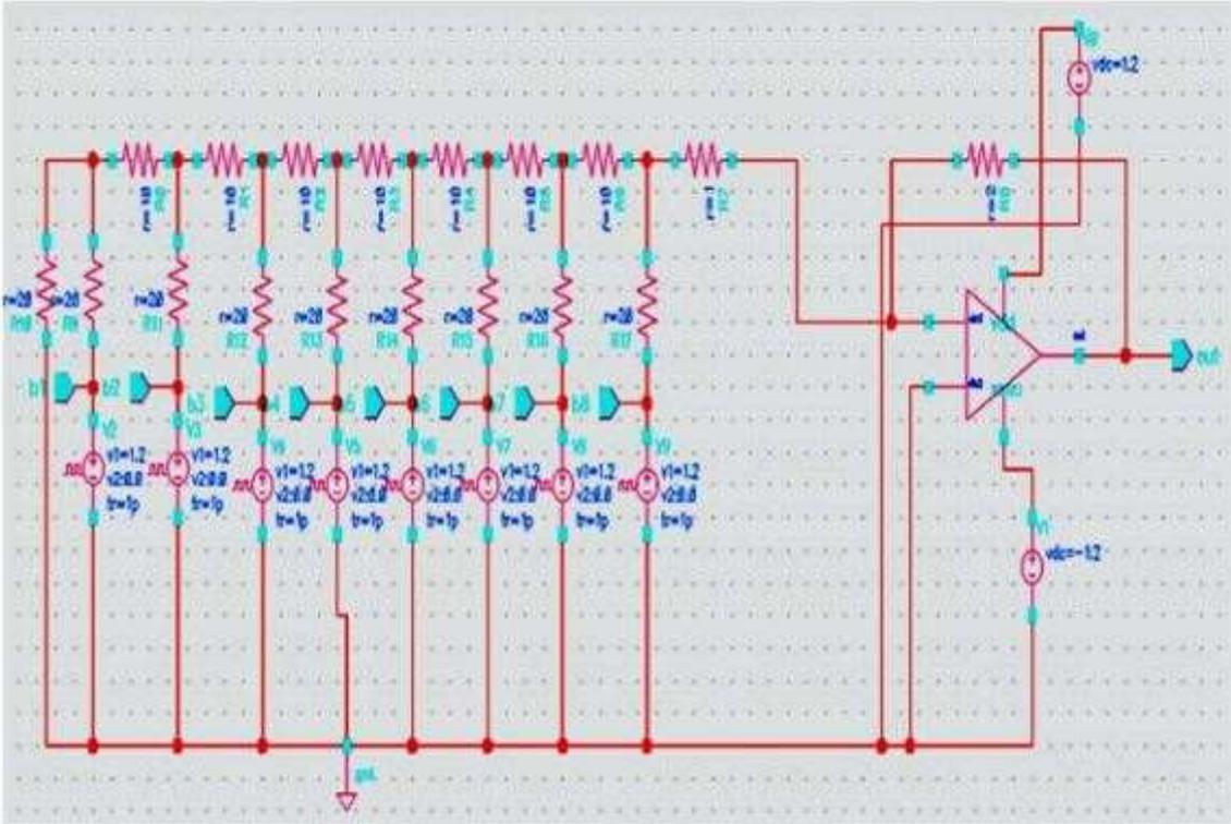
**Figure 3:** Circuit diagram of the Op-Amp based DAC
