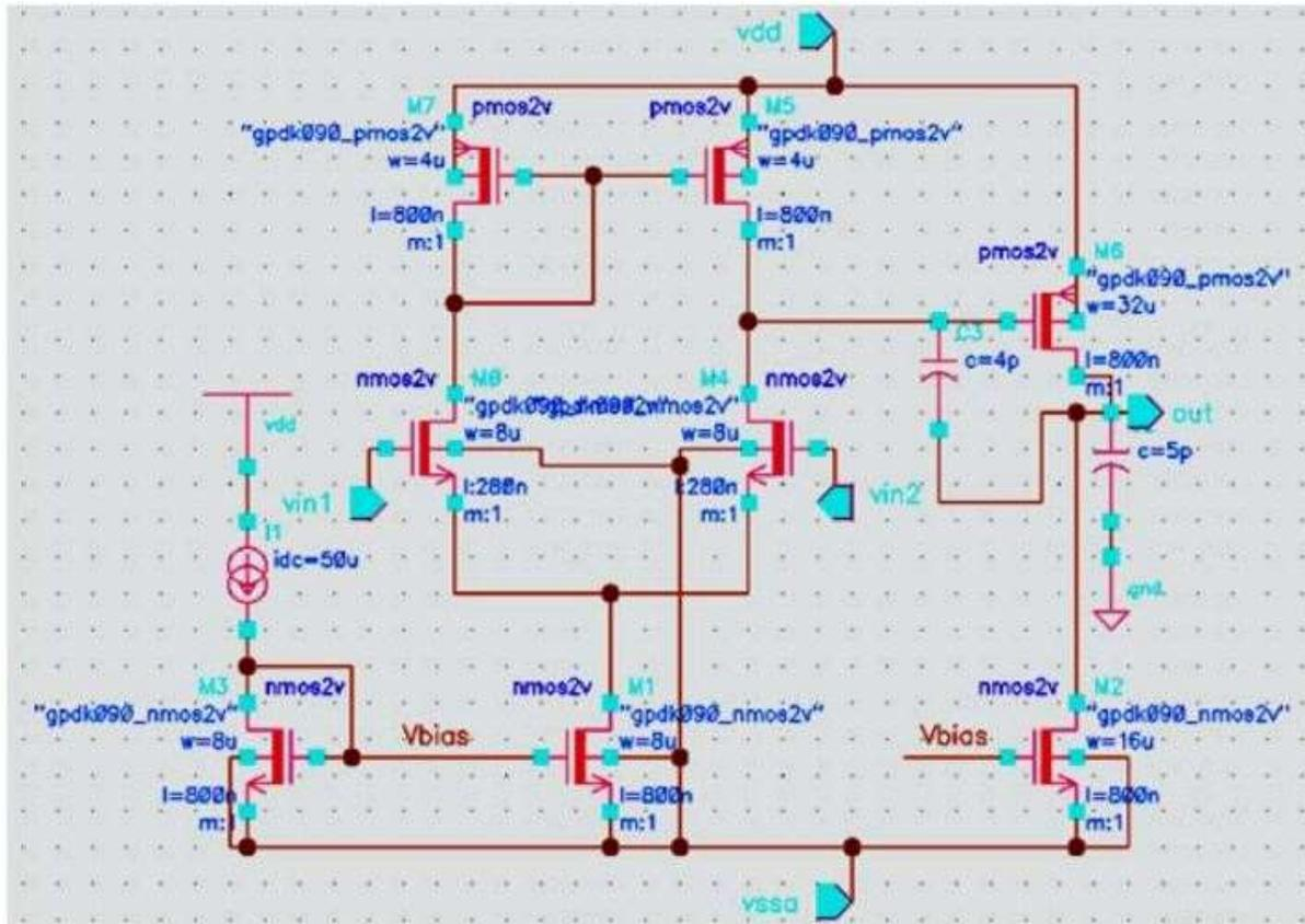
**Figure 4:** Circuit diagram of the proposed Op-amp for DAC
