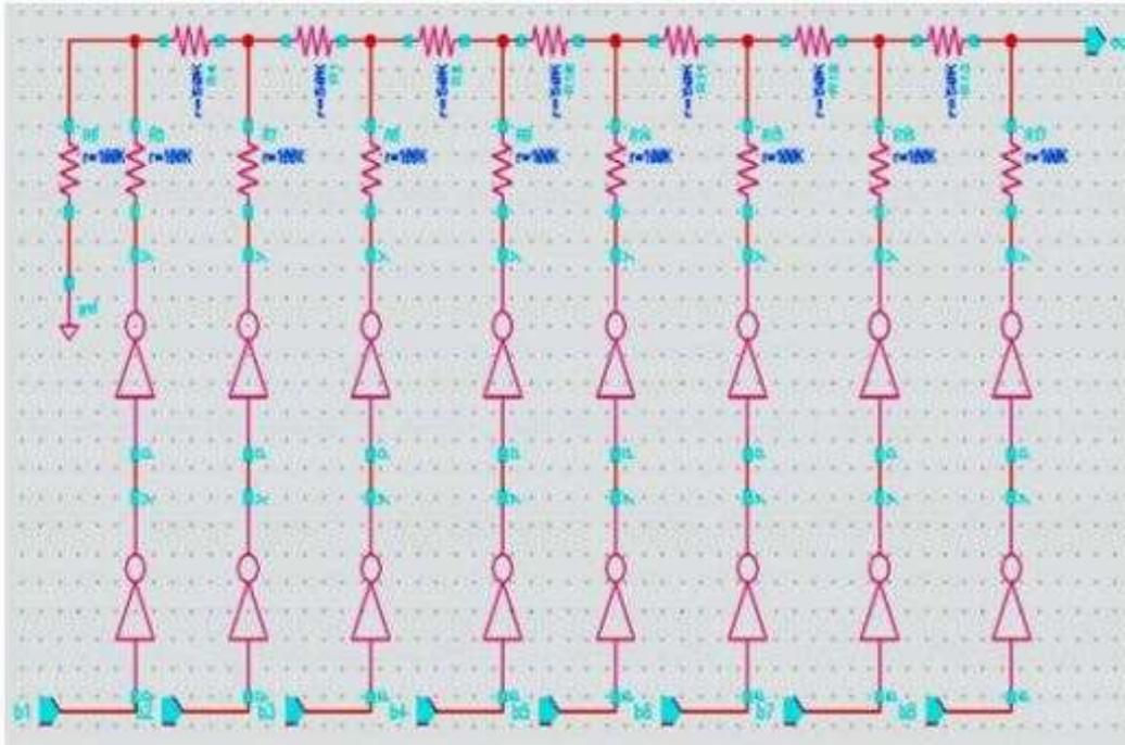
**Figure 2:** Circuit diagram of the R-2R ladder type DAC
