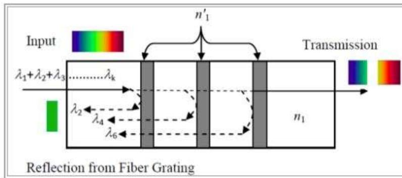
**Fig. 7: Simplified schematic of fiber Bragg refractometer sensor.**
