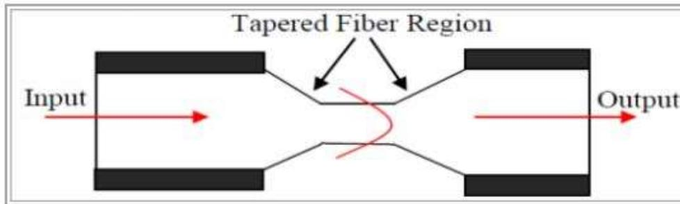
**Fig. 5: Tapered fiber optic sensor for RI measurement.**
