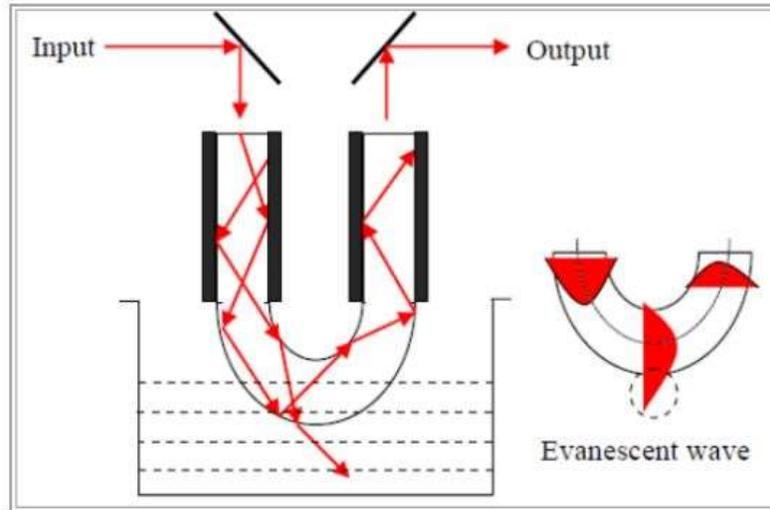
**Fig. 6: Simplified schematic of U-shaped bent fiber refractometer.**
