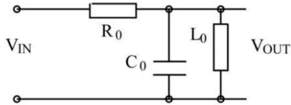
**Fig. 5: RLC band pass filter circuit**
