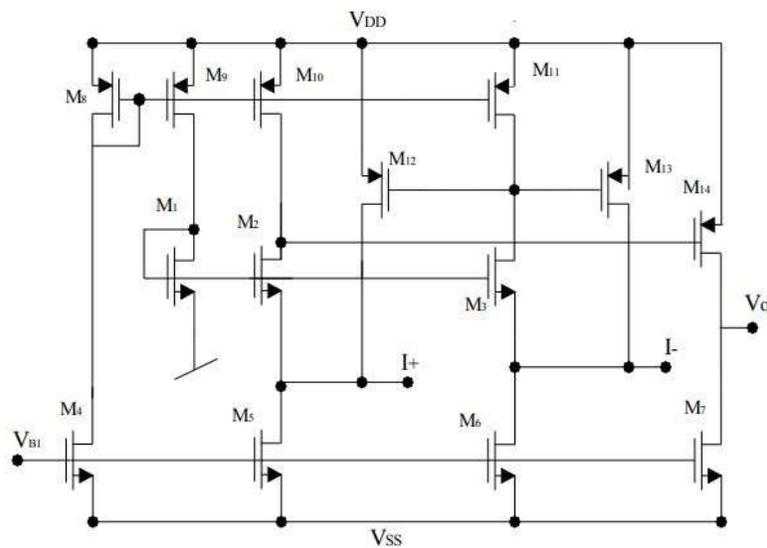
**Fig. 3: OTRA implementation using CMOS technology**
