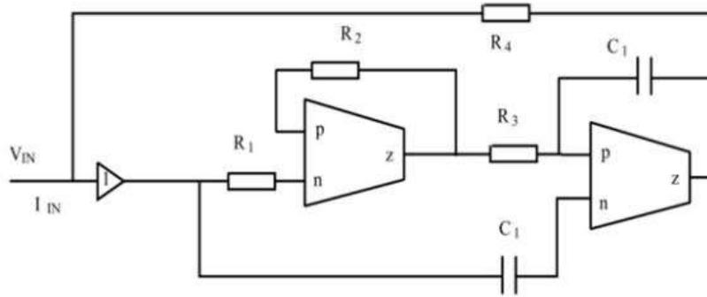
**Fig. 4: Simulation of grounded inductor using OTRA**
