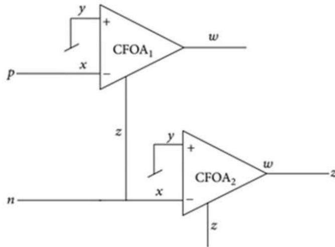
**Fig. 2: OTRA implementation using CFOAs**
