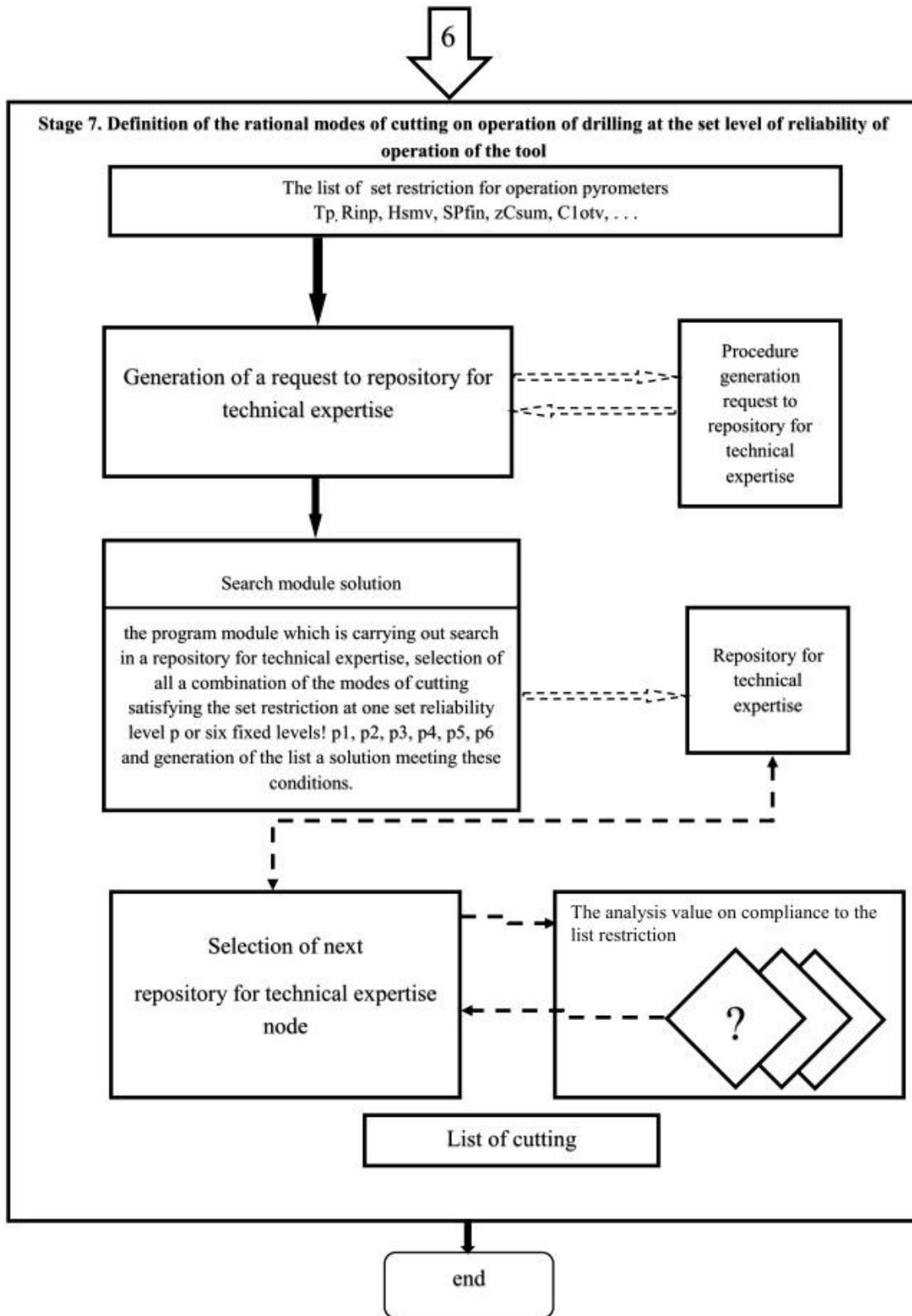
Figure 2. Sequence of Definition of the Modes of Cutting providing the set probability  $p$  trouble-free operation of the axial tool in the presence of the limiting factors.
