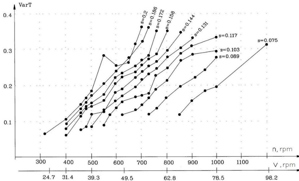
Figure 1. Dependence of a variation of firmness of drills on the cutting modes. Results of simulation modeling of processing of structural steel ( $\sigma_b=610$  MPa;  $HBo=2235$  MPa;  $VarHB=20\%$ ) pointed drills with plates from BK8
