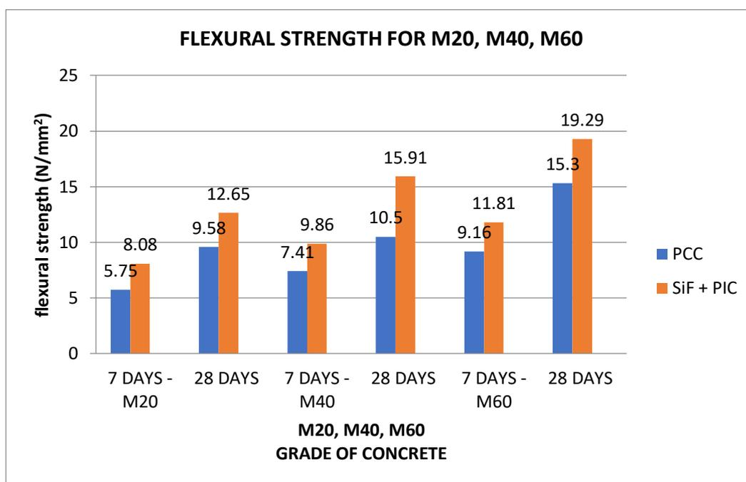
**Figure 5 Comparison Between Silica Fumes And Conventional Concrete**
