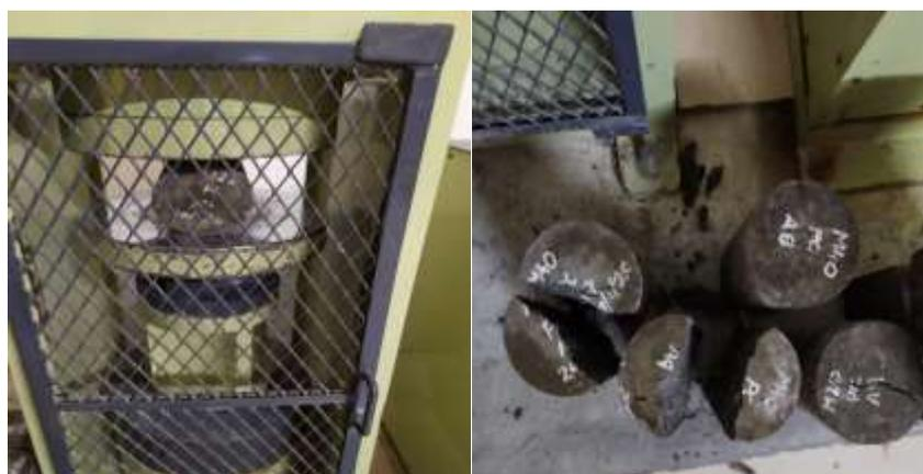
**Fig 6 Figure Showing Split Tensile Strength**
