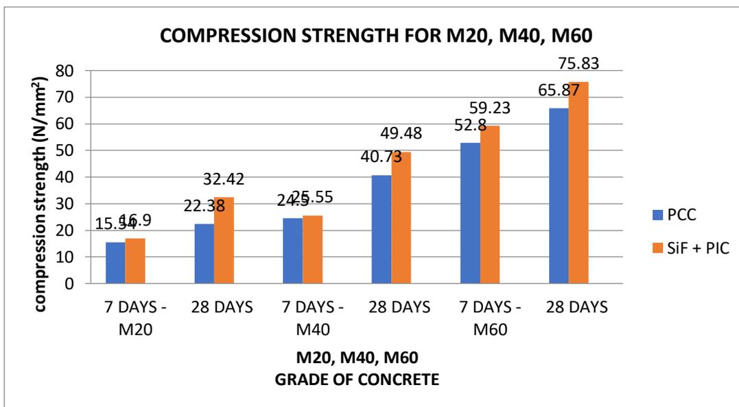
Figure 3 Comparison Between Silica Fumes And Conventional Concrete
