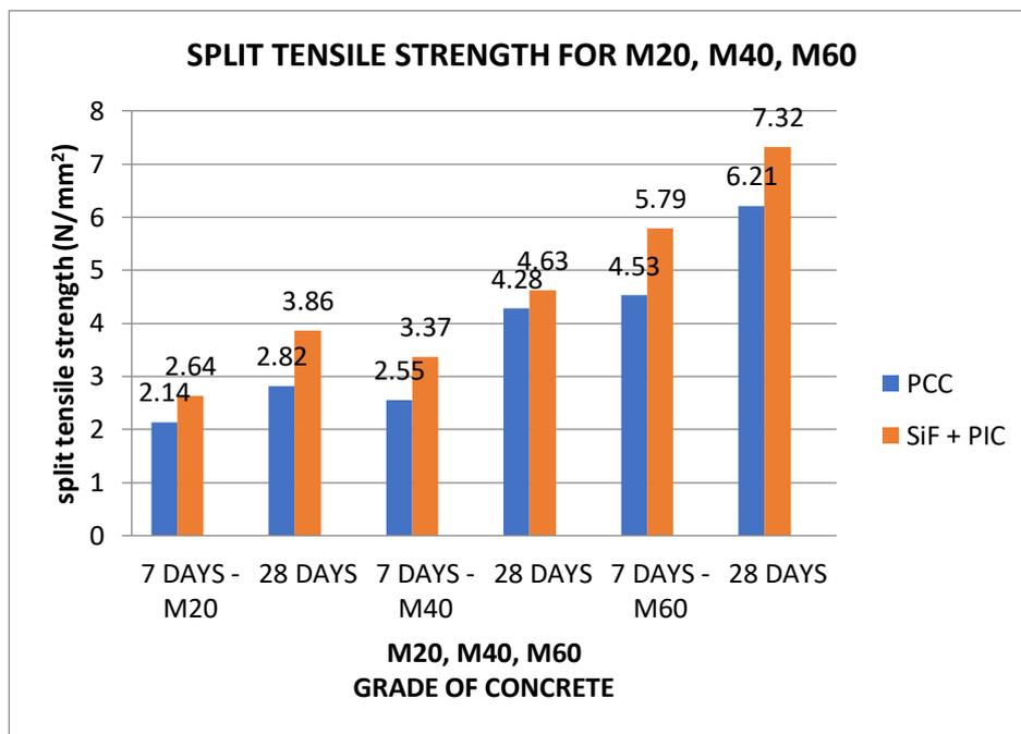
Figure 7 Comparison between silica fumes and conventional concrete
