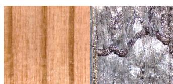
Figure 5: Normal and Burned surface surface of wood.
