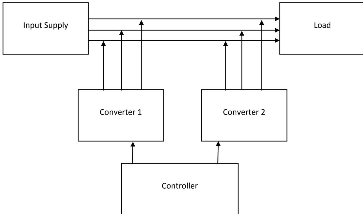
Figure 1: UPQC control Block diagram
