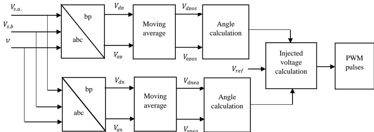
Figure 3: Series Active Power Filter
