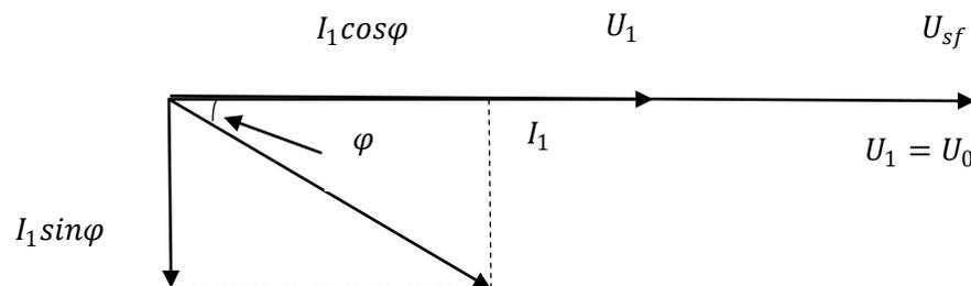
Figure 4: In-phase compensation Phasor diagram
