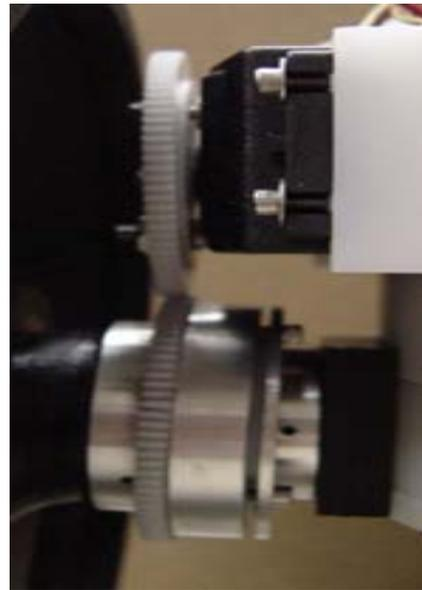
Figure 6: Nozzle gear assembly
