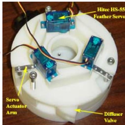
Figure 4: Diffuser Valve Assembly
