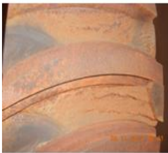
Blade crack at Root
