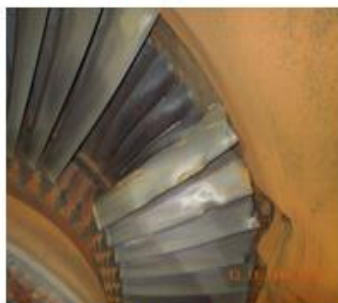
Damaged LP Rotor Final Stage Blades
