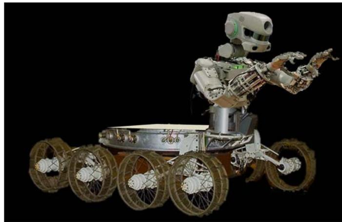
Fig. 14: The variant of the anthropomorphic robot of the Skybot f-850 project on a wheeled-walking chassis of moon rovers.
