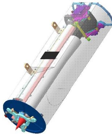
Fig.2: Reusable deep logging probe (RDLP).
