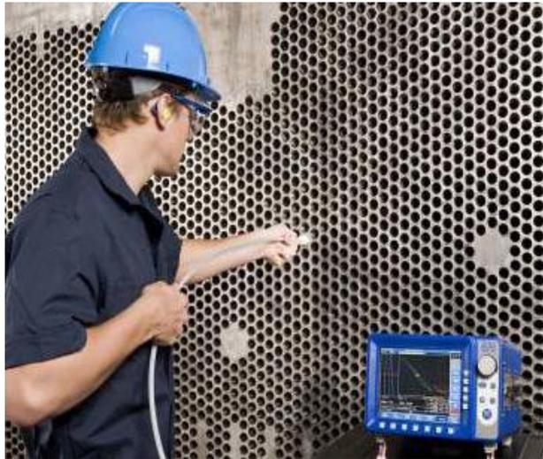
Fig.5: Eddy current test
