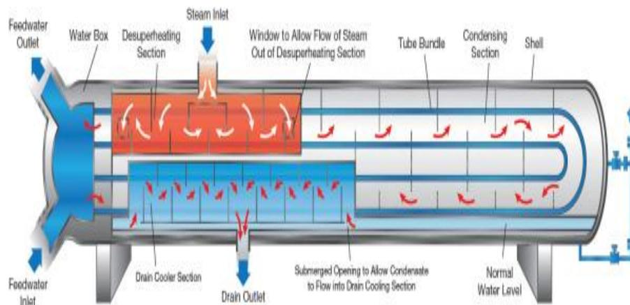
Fig.2: Different zones of Heater
