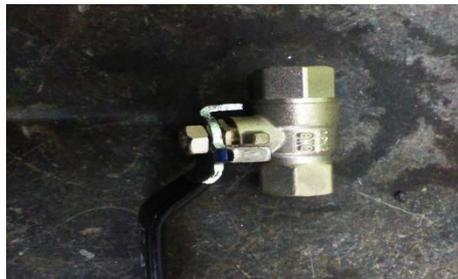
Flow Control Valves are fitted to all the distribution tubes. This valve is made of brass. Both the ends have stepped surface to insert hoses. A handle is provided to control the flow of oil in every valve.
