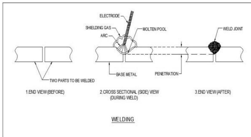
The operator needs to control the gap between the electrode tip and the work piece while moving the electrode along the joint.
