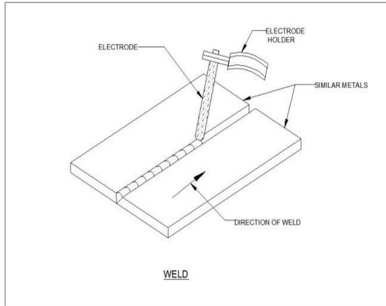
Welding is used for making permanent joints. It is used in the manufacture of automobile bodies, aircraft frames, railway wagons, machine frames, structural works, tanks, furniture, boilers, general repair work and ship building.
