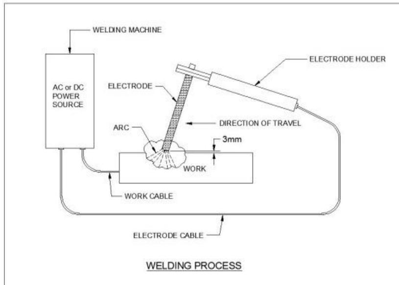
In the shielded metal arc welding process (SMAW) the 'stick' electrode is covered with an extruded coating of flux. The heat of the arc melts the flux which generates a gaseous shield to keep air away from the molten pool and also flux ingredients react with unwanted impurities such as surface oxides, creating a slag which floats to the surface of the weld pool. This forms a crust which protects the weld while it is cooling. When the weld is cold the slag is chipped off.
