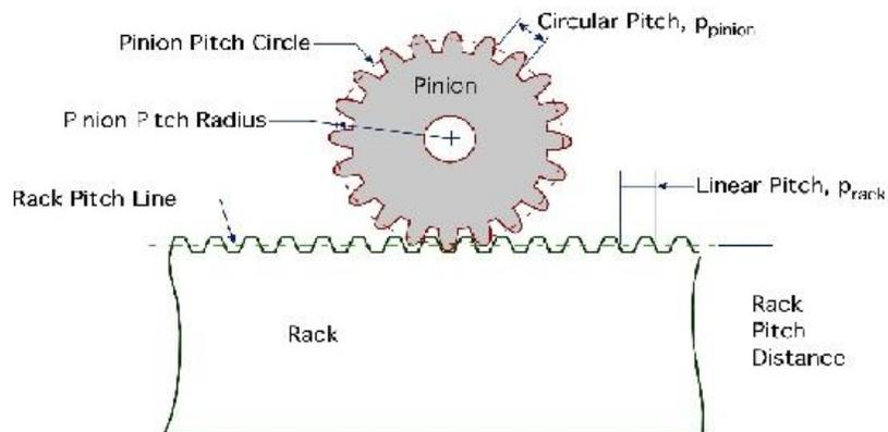
A rack and pinion is a type of linear actuator that comprises a pair of gears which convert rotational motion into linear motion. A circular gear called “the pinion” engages teeth on a linear “gear” bar called “the rack”; rotational motion applied to the pinion causes the rack to move, thereby translating the rotational motion of the pinion into the linear motion of the rack.
