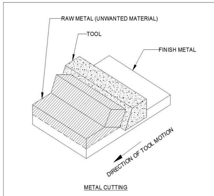
Cutting processes work by causing fracture of the material that is processed. Usually, the portion that is fractured away is in small sized pieces, called chips. Common cutting processes include sawing, shaping (or planing), broaching, drilling, grinding, turning and milling. Although the actual machines, tools and processes for cutting look very different from each other, the basic mechanism for causing the fracture can be understood by just a simple model called for orthogonal cutting.
