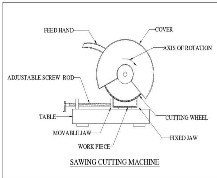
The circular saw blades used with a cold saw are often constructed of high speed steel. Steel blades of this type are resistant to wear even under daily usage. The end result is that it is possible to complete a number of cutting projects before there is a need to replace the blade. High speed steel blades are especially useful when the saws are used for cutting through thicker sections of metal.
