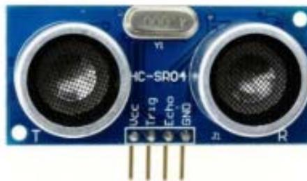
**Figure 4:** HC-SR04 Ultrasonic sensor type [7].
