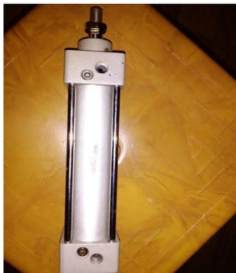
Stroke length: Cylinder stoker length 160 mm = 0.16 m
