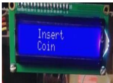
Fig. 5. Message in idle state (Door Locked)
