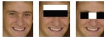
Figure 5. Examples of Haar Feature .Area of White and black region are multiplied by their respective weights and then summed in order to get the HAAR Feature Value
