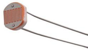
Fig. 2. Typical LDR Sensor
