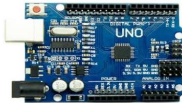
Figure 5 Arduino UNO Board
