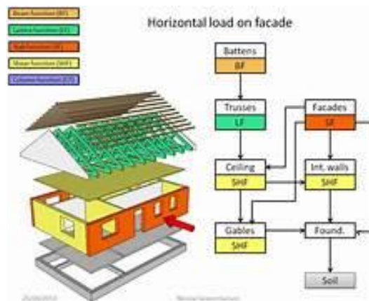
Fig 2. Process of Structural Analysis
