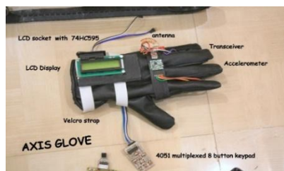
Fig. 3. Glove made with accelerometer to control motor
