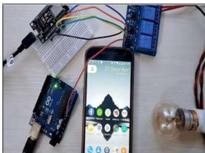
Fig.8: Light initially OFF when no voice command is given
