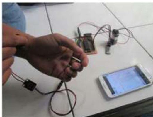
Fig. 8. The experimental test of the proposed heartbeat meter.
