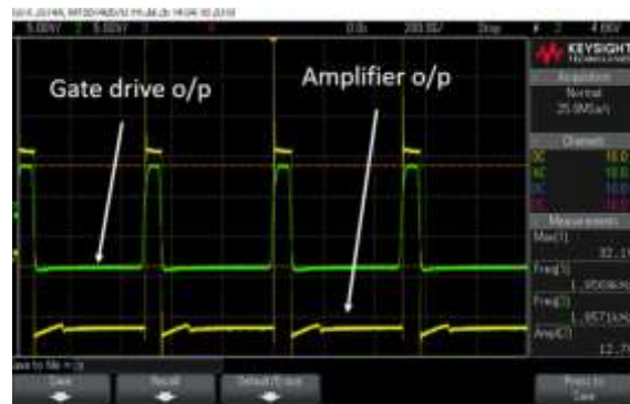
Fig.27: Output waveform of asymmetrical bridge power amplifier (Duty cycle=25%).
