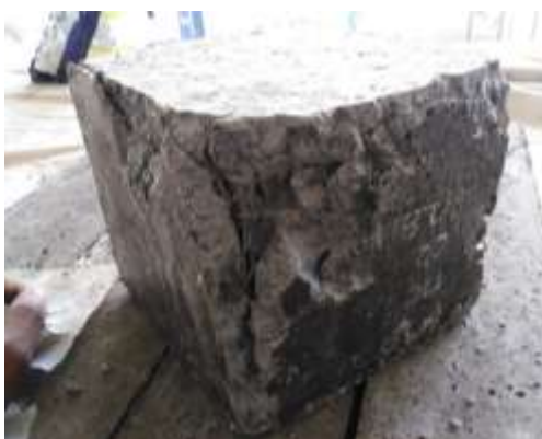
Figure 10. tested cube specimen with wire mesh
