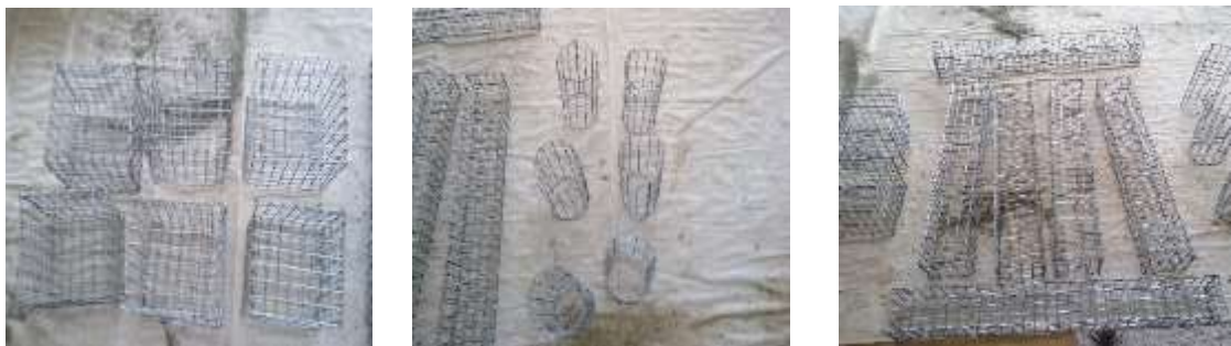
Figure 2. specimen shape of steel wire mesh for cube, prism and cylinder
