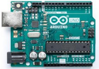
Figure 1: Arduino Uno Rev ATmega 328
