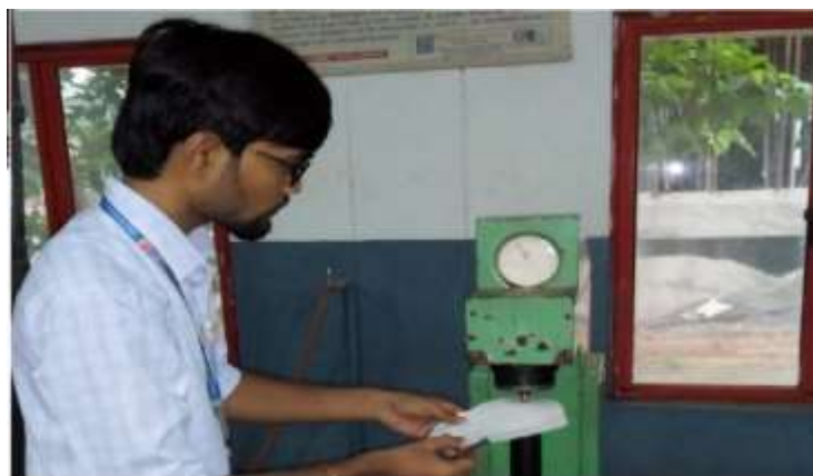
Figure 8: Rockwell hardness tester
