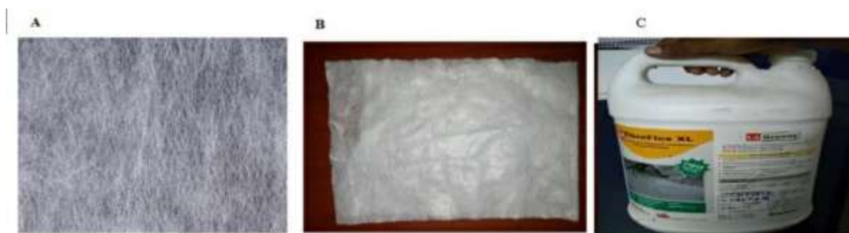
Figure 1: Raw materials A) Non-woven fabric B) Layers of Non-woven fabric C) Acrylic polymer binder
