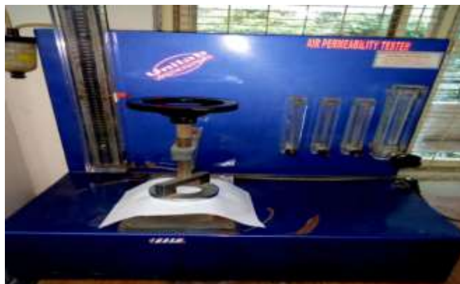
Figure 7: Air permeability test apparatus
