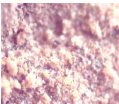
Figure 7a: The structure (x100) of the sample - samples of the historic masonry mortar wall of the madrasah of Abdulazizkhan
