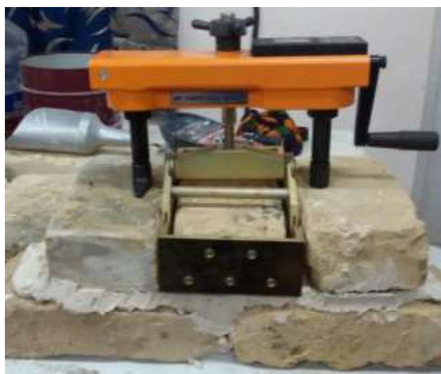
Figure 10: Photo taken from the process of testing to determine the adhesion strength of the mortar to the masonry bricks.
