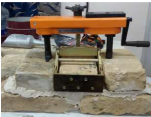
Figure 10: Photo taken from the process of testing to determine the adhesion strength of the mortar to the masonry bricks.
