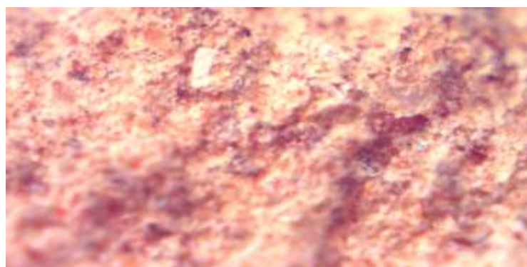
Figure 9: The structure (x100) of a sample of a brick of the upper part of the wall mausoleum of Ismail Samaniy
