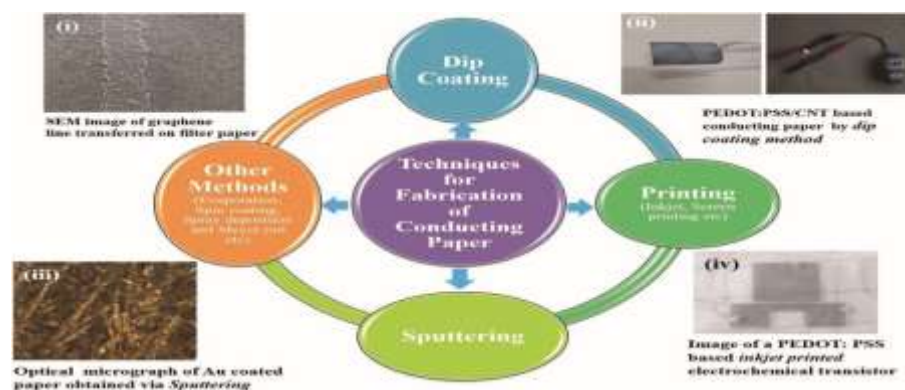
Figure 4. Fabrication of CP via different technique. Reproduced with permission. a) Copyright 2016, AIP Publishing. b) Copyright 2017, IOP Publishing. c) Copyright 2013, Wiley-VCH. d) Copyright 2015, RSC Publishing [85, 86].
