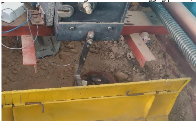
Fig. 4. The process of digging the components of solid waste at the bench of physical modeling with the openers operating position.
