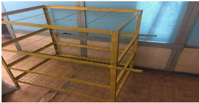
Fig. 1. General view of the bench for determining the fractional composition of solid waste
