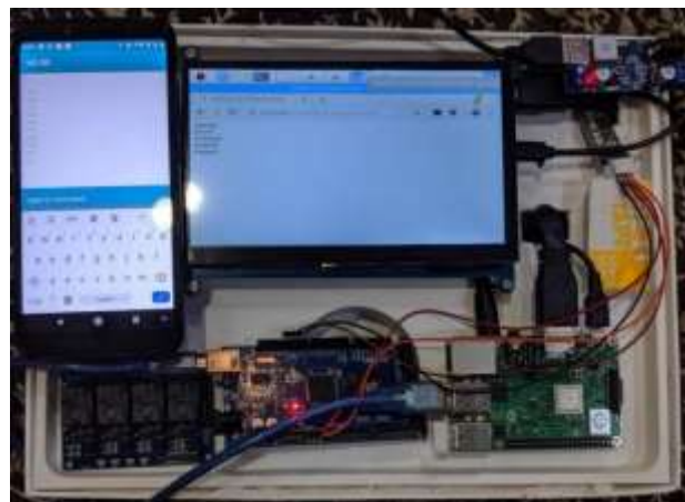
Figure 8: Showing mobile app-controlled automation with admin webserver live monitoring system
