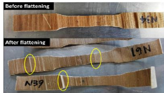
Figure 5: Cracking Happened on the Perpendicular Oriented Samples During Flattening Process, the Circled Parts Indicate the Cracks
