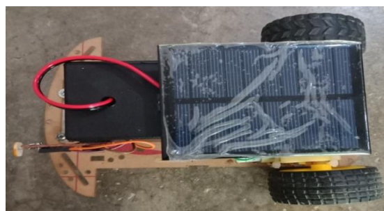
Figure 3: The design of a-watt solar module on a robot car with interface control system from android
