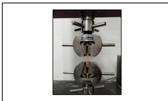
Figure 2: Tensile test PMMA-Silicone SDL specimen with UTM (Tensilometer, AND, RTF – 1350, Japan)
