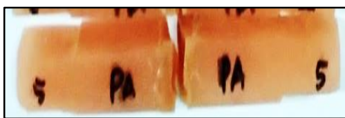
Figure 4: Cohesive failure mode of PMMA-heatpolymerized silicone SDL after molloplast primer adhesive
