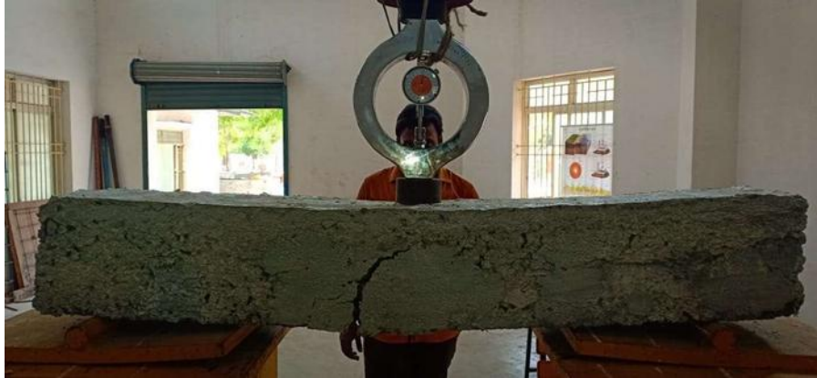
Fig. 2: Yield failure of Beam (Bamboo Reinforcement)
