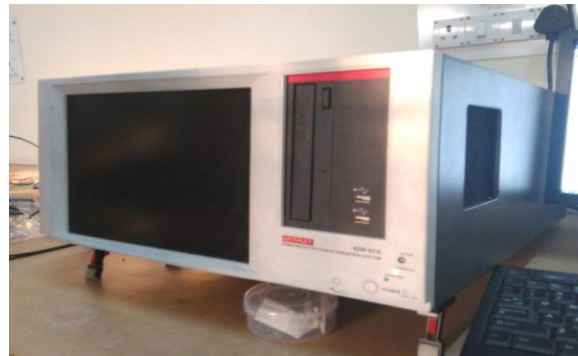
Fig.8: The Electrometer SCS-4200 (Keithley, USA). [By Courtesy: Semiconductor Research Lab, GKV, Haridwar]
