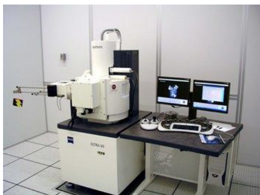
Fig.3: Field emission scanning electron microscopy (FE-SEM) (Zeiss Ultra60). [By Courtesy: Institute Instrumental Centre, IIT Roorkee]
