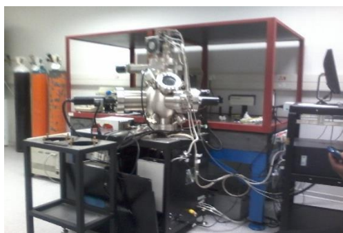
Fig.5: The Photoluminescence Spectrometer with He-Cd Laser of 325 nm. (By Courtesy: Department of Physics, University of Free State, Bloemfontein, SA)
