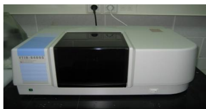
Fig.6: The FTIR 8400S Fourier transform infrared spectrometer of Shimadzu, Japan. (By Courtesy: Department of Chemistry, GKV Haridwar)
