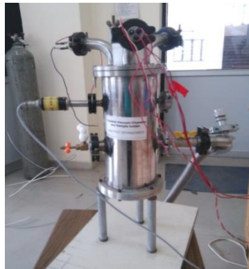
Fig.9: Gas sensing measurement chamber (By Courtesy: Semiconductor Research Lab, Department of Physics, GKV Haridwar)
