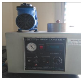
Fig.16: Spin coater (Metrex Scientific Instruments Private Limit India). (By Courtesy: Semiconductor Research Lab, Department of Physics, GKV Haridwar)
