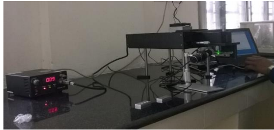
Fig.7: The RIRM–LP Raman spectrometer of RI Instruments & Innovation, India. (By Courtesy: Manufacturing Unit of RI Instruments & Innovation, India)
