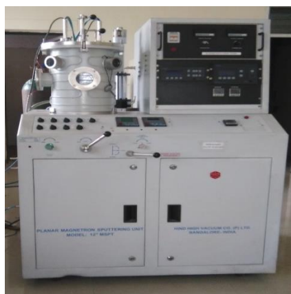
Fig.17: The Planar Magnetron RF/DC Sputtering Unit Model 12" MSPT (Hind High Vacuum Co. (P) Ltd. Bangalore, India).
