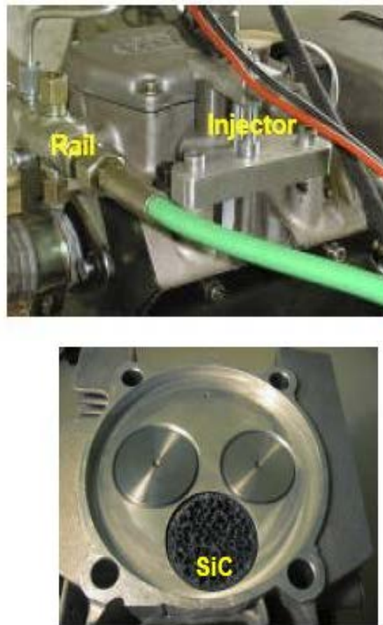
Figure 10 Top and bottom view of the PM-engine head with SiC reactor mounted in space between valves
