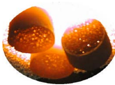
Figure 3: View of the SiC reactors under thermal test for engine application
